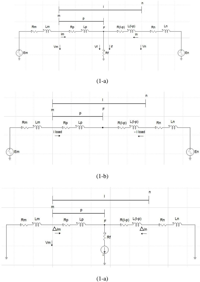
**Figure 1:** Linear circuit of transfer system transient model. (1-a): the circuit in error condition. (1-b): the circuit in loading condition. (1-c): the circuit of network error component
