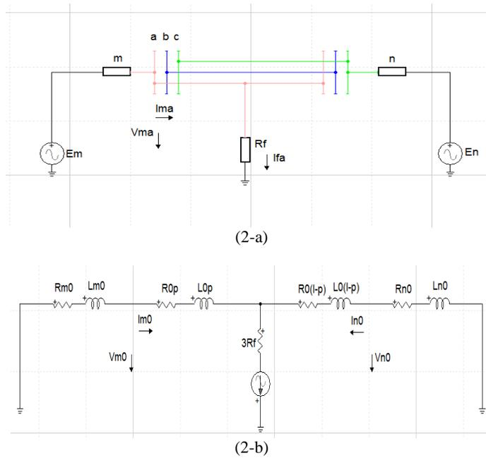
**Figure 2:** The circuit of three phase transfer system in the condition of phase to ground fault (2 – a): the circuit in error condition. (2 – b): linear circuit in zero sequence
