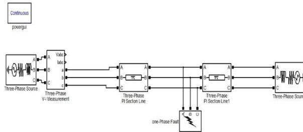
Figure 4: Simulated RL three phase transfer line by MATLAB in error condition
