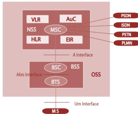
Figure 7 GSM architecture.
