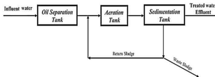
**Figure 2.** Schematic of BTL effluent water treatment process
