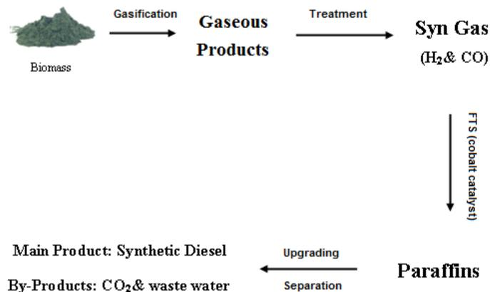
**Figure 1.** Schematic of biomass to liquid fuels process
