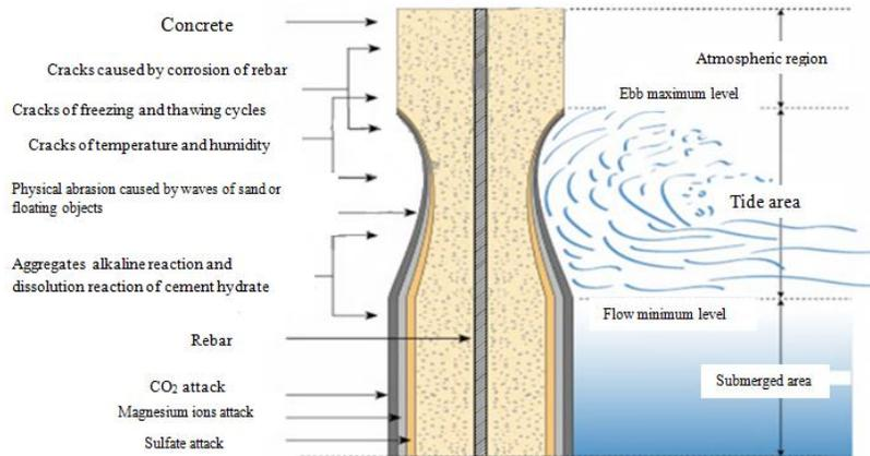
**Figure 2:** possible collapses and their place in a concrete column in seawater
