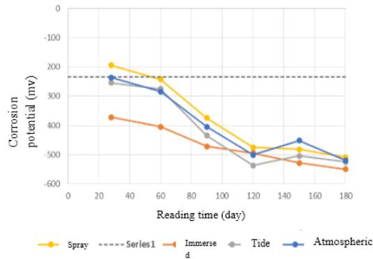
Figure 2: The corrosion potential of samples A2 in different circumstances, at the age of 28, 60, 90, 120, 150 and 180 days
