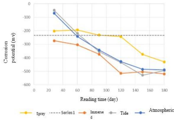
Figure 1: The corrosion potential of samples A1 in different circumstances, at the age of 28, 60, 90, 120, 150 and 180 days
