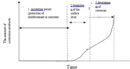
**Figure 1:** The model proposed by Tuutti, the corrosion of reinforcing steel in concrete [8]
