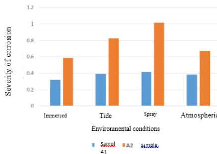
Figure 3: The results of corrosion current density for various environmental samples at the age of 180 days
